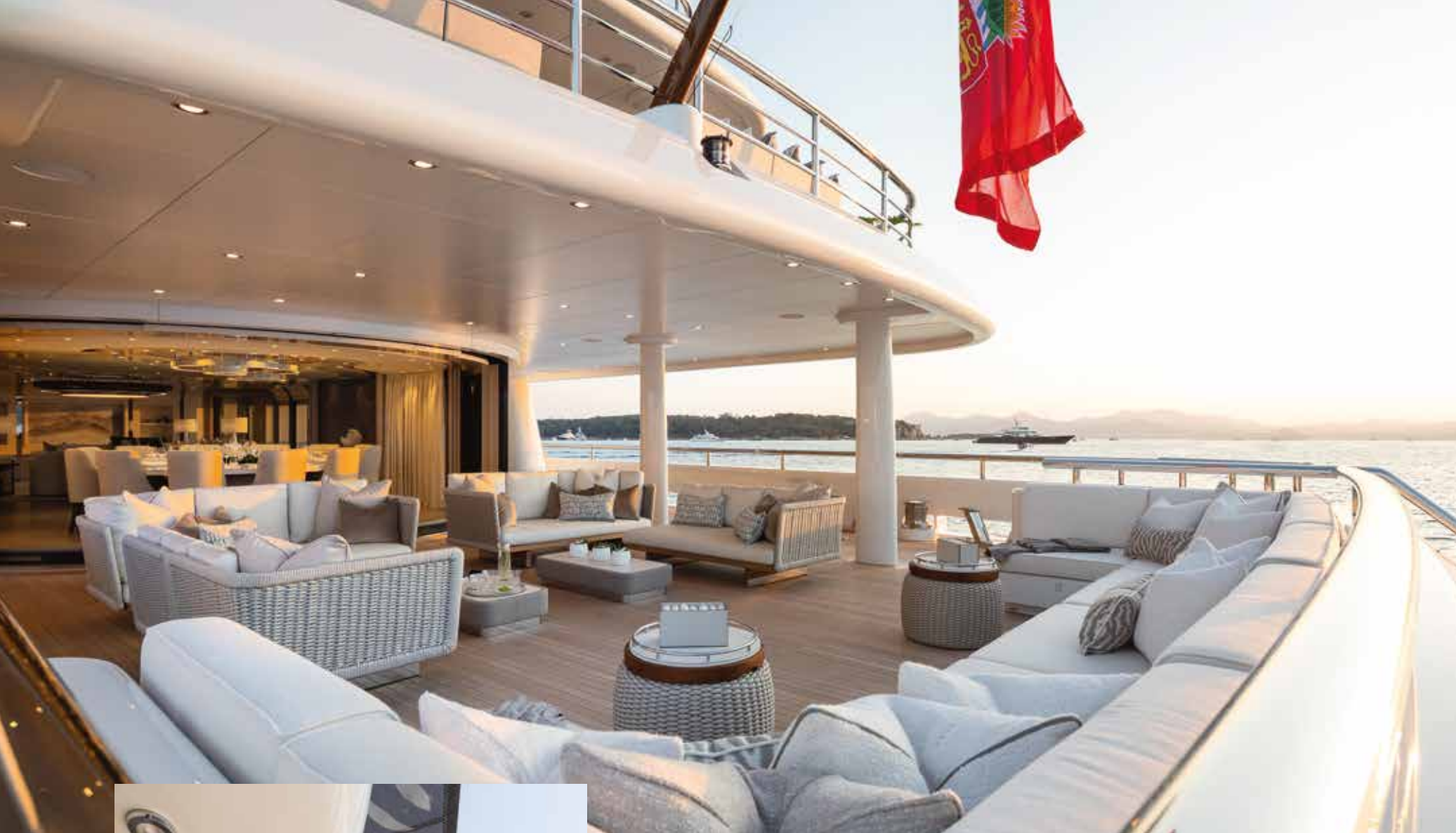
The transom was stretched by 50cm to comfortably fit sun loungers on the platform and spa facilities inside (above and below). The owner also altered the sundeck design by removing the helipad, leaving plenty of room for relaxation (bottom left and right). The vast main deck aft (left) needed no adjustment
